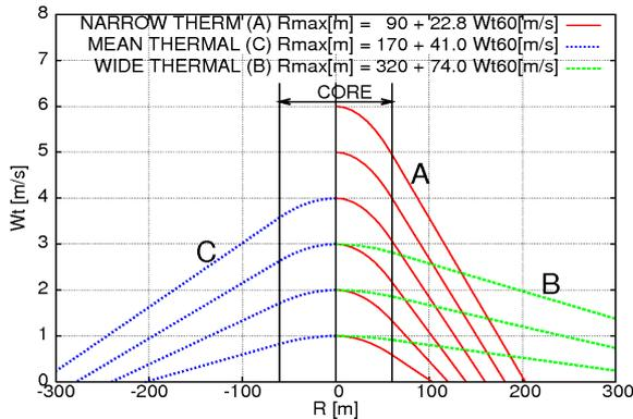
Fig. 2 Assumed lift distribution in model thermals.
